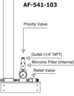
AF-541-103 Maximum CFM: 12 \*Typical Cartridge Life: 16000 CF Cartridge: X542423 Dimensions: 12"W x 36"H x 5"D
