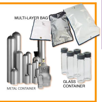
There are various means for capturing, containing, & analyzing Air-&-Gas. Much is determined by the gas, the pressure, timing, and the analytes.
